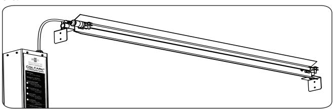
Optional vertical support adds strength to the tube framing and prevents sagging on installations with two or more lamps per tubing length.
