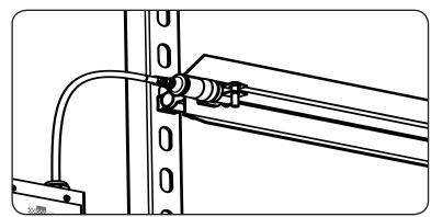
Optional vertical support adds strength to the strut framing and prevents sagging on installations with two or more lamps per strut length.
