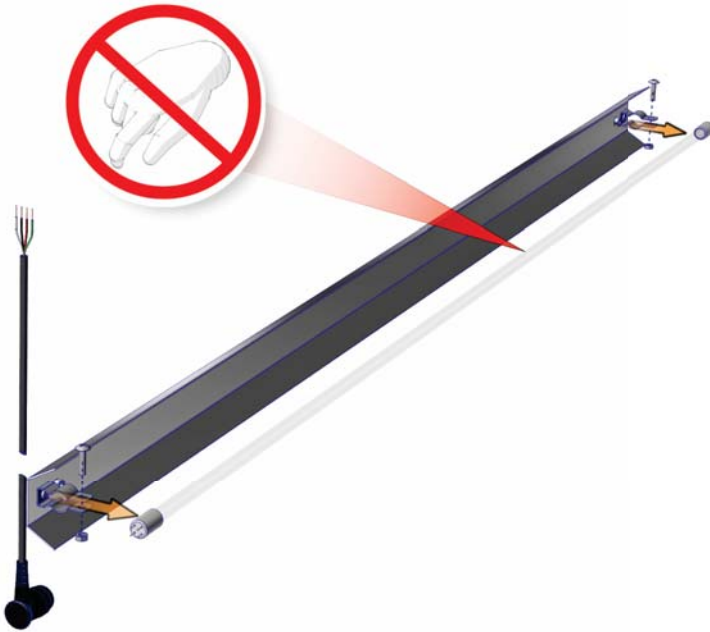
Figure 15: Removing UVC lamp from fixture
